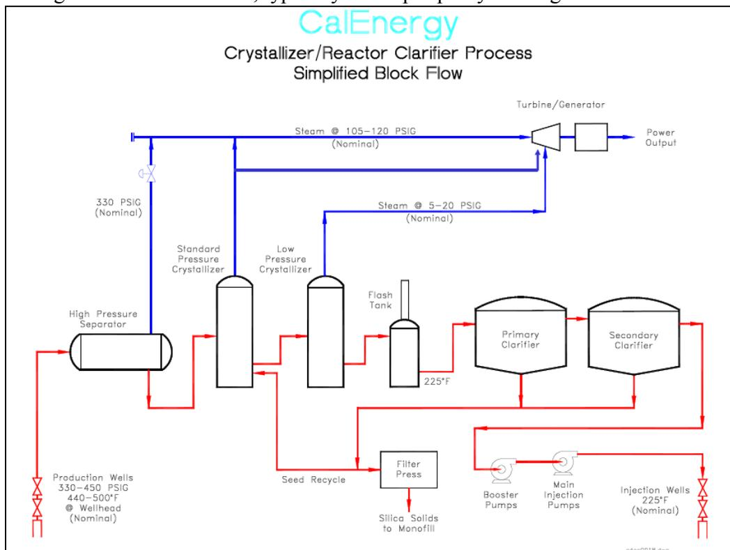
Figure 5. Triple flash brine and steam process as employed by CalEnergy (from CalEnergy public talk)
